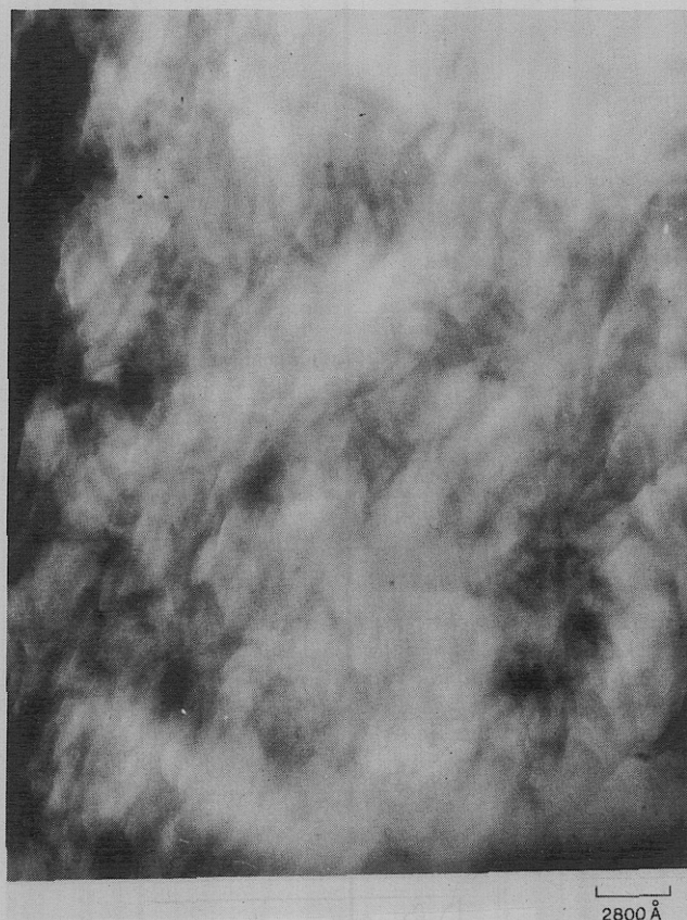
Figure 8. Typical area of tagged PE of M_v = 2.9 \times 10^6 in untagged PE.
